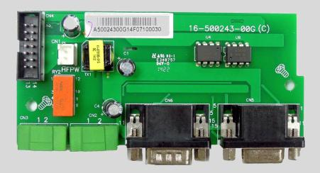
This accessory is applicable only to the 48VDC models of HS and MS series inverter. It is a required component to be installed in every unit of a parallel system. A parallel kit includes:
